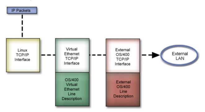
IP traffic initiated by the logical partition goes from the Linux network interface to the virtual i5/OS interface. If the virtual interface is associated with the external interface, the IP packets can continue on to the external interface and towards its destination.
