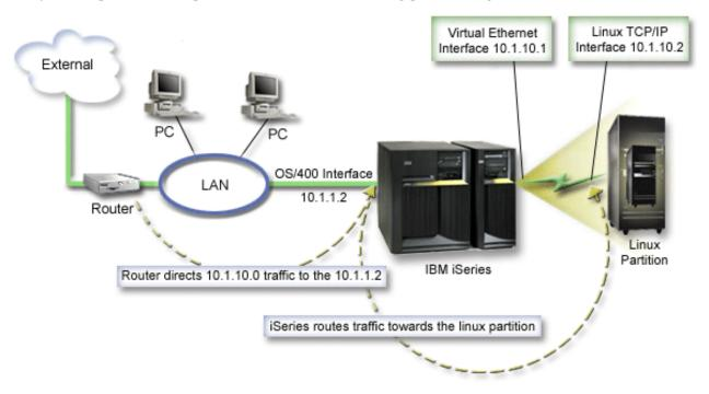
The existing TCP/IP interface (10.1.1.2) connects to the LAN. The LAN is connected to remote networks with a router. The Linux TCP/IP interface is addressed as 10.1.10.2 and the virtual Ethernet TCP/IP interface as 10.1.10.1. In i5/OS, if you turn on IP Datagram Forwarding, the iSeries will route the IP packets to and from the logical partition. When you define your Linux TCP/IP connection, the router address must be 10.1.10.1.
