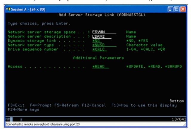
On the Add Network Server Storage Link (ADDNWSSTGL) display, the value you enter in the Dynamic storage link field can be either \*YES or \*NO. To display the Access option, press the F9 key. If multiple Linux partitions share disks, the partitions must access (that is, mount) the disks from Linux with read-only access.
