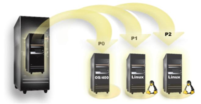
(Pre-V5R3 diagram) Linux is not supported on a primary partition. Additional information on software function can be found at i5/OS logical partition function by release.
