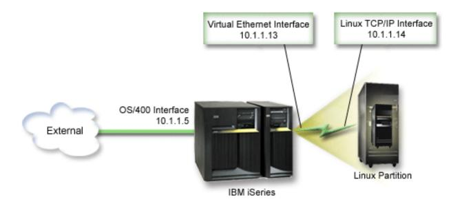
In this example, a contiguous block of four IP addresses is used, which is 10.1.1.12 - 10.1.1.15. Since it is a block of four IP address, the subnet mask for these addresses is 255.255.255.252. To configure a setup similar to this, use the following instructions:
