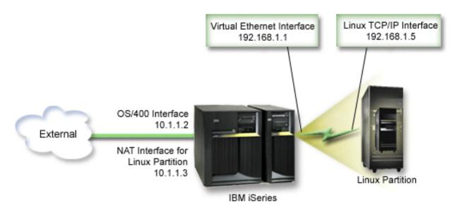
In this pre-V5R3 example, any existing TCP/IP traffic for the iSeries hosting partition runs over the 10.1.1.2 interface. Since this is a static map scenario, the inbound traffic gets translated from the 10.1.1.3 interface to 192.168.1.1 interface. The outbound traffic gets translated from the 192.168.1.1 interface to the external 10.1.1.3 interface. The logical partition uses the virtual interface (192.168.1.1) and its own 192.168.1.5 interface to communicate with the server.
