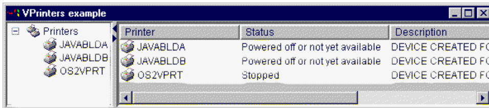
Figure 4: Using AS400ExplorerPane with a VPrinters object
