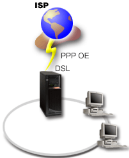
Figure 3. Connect your iSeries server to an ISP with PPPoE
